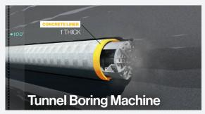
2 While the boring machine moves forward, it lifts segments of a 1-foot-thick reinforced concrete liner into place. Grout completes the seal.
