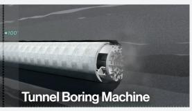
1 The tunnel would be bored through rock as much as 100 feet below the lake bed, using an apparatus called a Tunnel Boring Machine.
