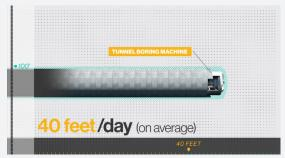
3 Like a giant mechanical earthworm, the tunnel boring machine would move an average of 40 feet a day, five days a week. At that rate, it's expected to take about two years to make its way across the full 4.1 miles under the Straits.
