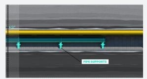
4 Pipe segments would be coated and welded in an onshore staging area. Supports with rollers will be bolted along the tunnel wall, and the pipe pushed along that roller system—one long segment at a time.
